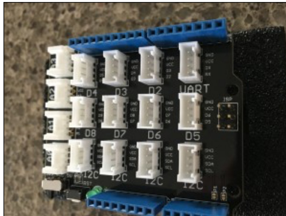
FIGURE 2-2: The Arduino Uno Grove base board.
