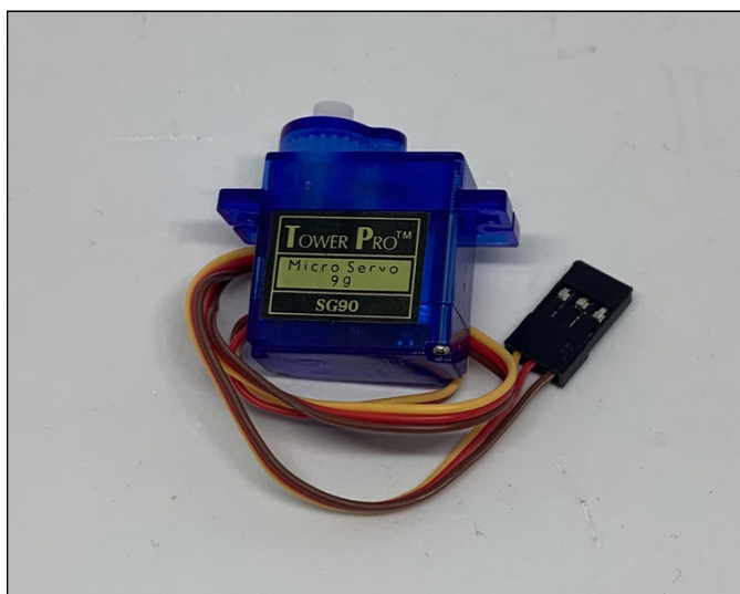
FIGURE 2-3: The SG90 micro servo motor.
