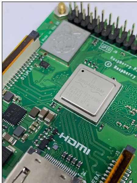
FIGURE 4-1: The Raspberry Pi processing chip containing the Videocore-IV.
