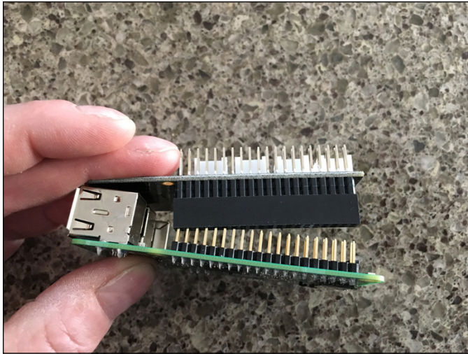
FIGURE 1-6: Aligning the Pi2Grover board on the Raspberry Pi.
