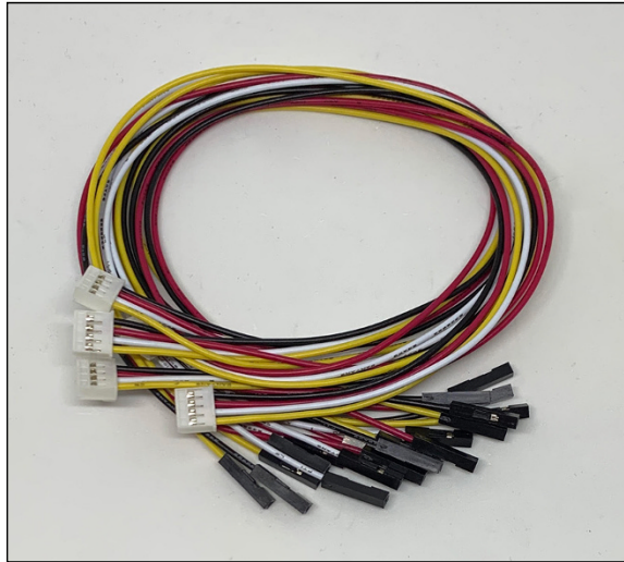
FIGURE 2-13: Grove male header cables.
