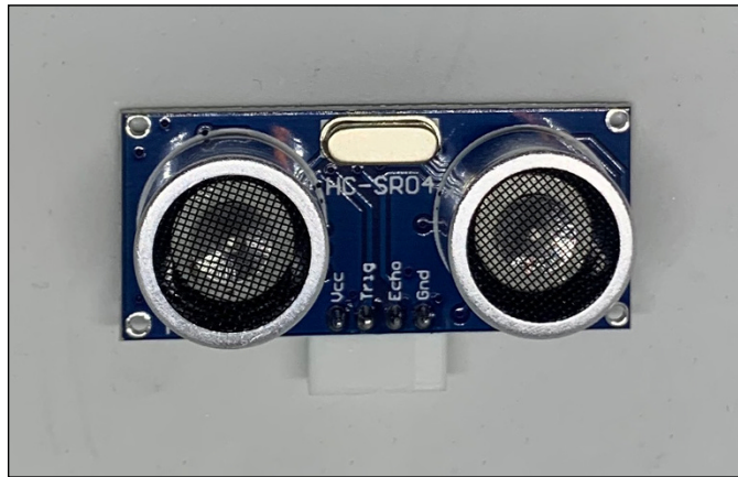
FIGURE 2-8: An ultrasonic distance sensor.
