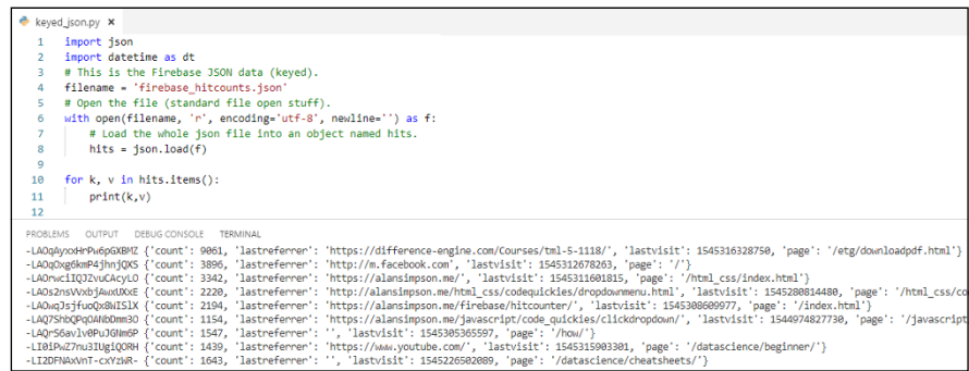
FIGURE 2-5: Output from looping through and displaying keys and values from sub-dictionaries.
