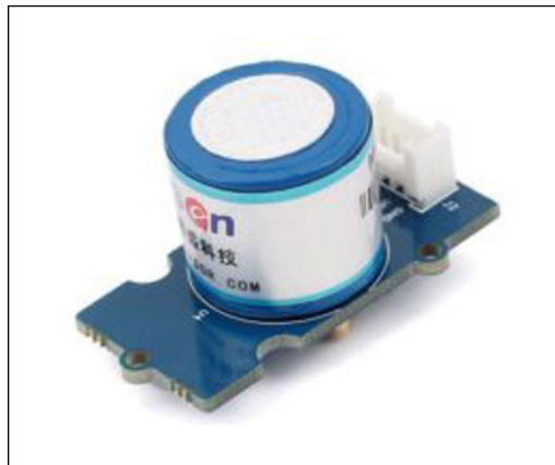
FIGURE 3-6: The Grove oxygen sensor.
